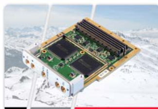
New ADC512 Analog-to-Digital Converter FMC Card Combines 3 GHz Sampling Rates and up to 6 GB/s Data Throughput
